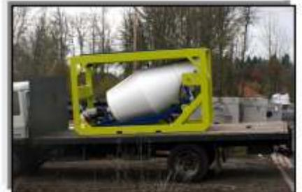
The C.U.B.E.® comes standard with a 91 CM by 3 meters sand and gravel conveyor that can be top-loaded by a skid steer. An integrated water and cement loading system allows for easy on-site batching at 7 plus meters per hour. Because it is UNIVERSAL, you can find several ways to save money using the C.U.B.E.®. to batch concrete.
